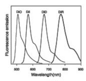
Normalized fluorescence emission spectra of DiO, DiI, DiD, and DiR bound to phospholipid bilayer membranes.
