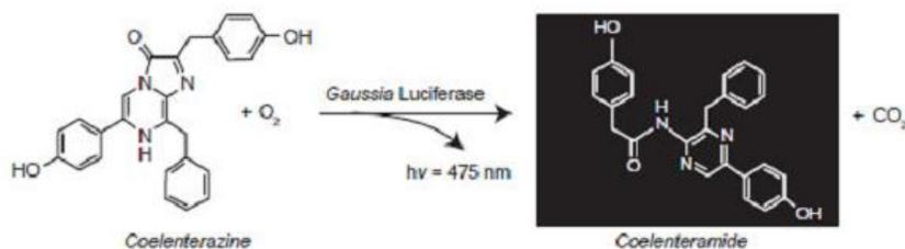
**Figure 1. The Photo-oxidation catalyzed by *Gaussia* Luciferase**
